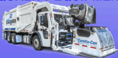
AUTOMATED FRONT LOADER (AFL)
